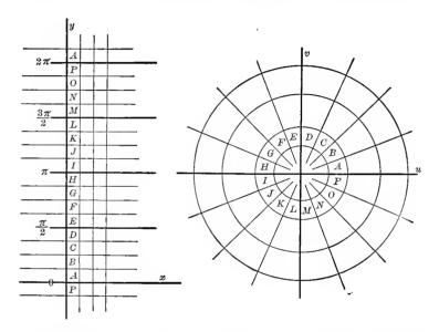
of straight lines parallel to the axis of x, dividing that plane into strips of equal width. To any curve in the w-plane which does not meet the line just drawn, will correspond in the z-plane an infinite number of curves, of which there will be one in each strip.
