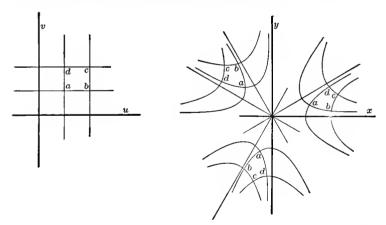
Prob. 8. If  $w = z + \frac{1}{z}$ , show that circles in the z-plane having a common center at the origin transform into confocal ellipses.
