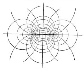
The velocities are everywhere, except at the points  $\pm a$ , finite and determinate. If the circles  $r_1/r_1 = \text{const.}$  be taken as the stream-lines, each of the points  $\pm a$  is a "vortex-point." If the circles  $\theta_1 - \theta_2 = \text{const.}$  be taken as the stream-lines, one
