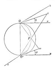
length to unity. Construct tangent planes at at O and O'. Draw in the tangent plane at O rectangular axes Ox and Oy; and in the other plane draw as axes O'u, parallel to Ox and measured in the same direction, and O'v parallel to Oy but measured in a contrary direction. Join any point z in the plane xOy to
